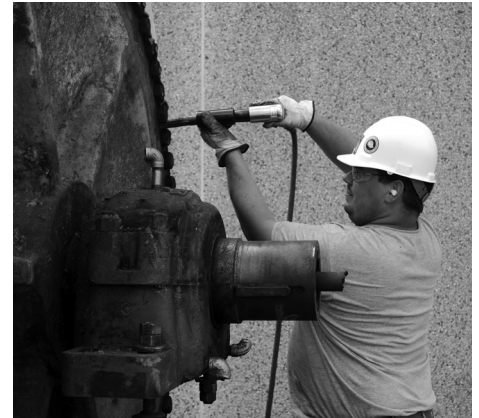
City Forest Paper Co. of Ladysmith, Wis., donated a paper machine to the Eastern Training Center in Kaukauna, Wis. Members disassembled the parts, sandblasted and painted the machine so apprentices could reassemble it as part of their training. Pictured is Cory Conard, Local 1056.
