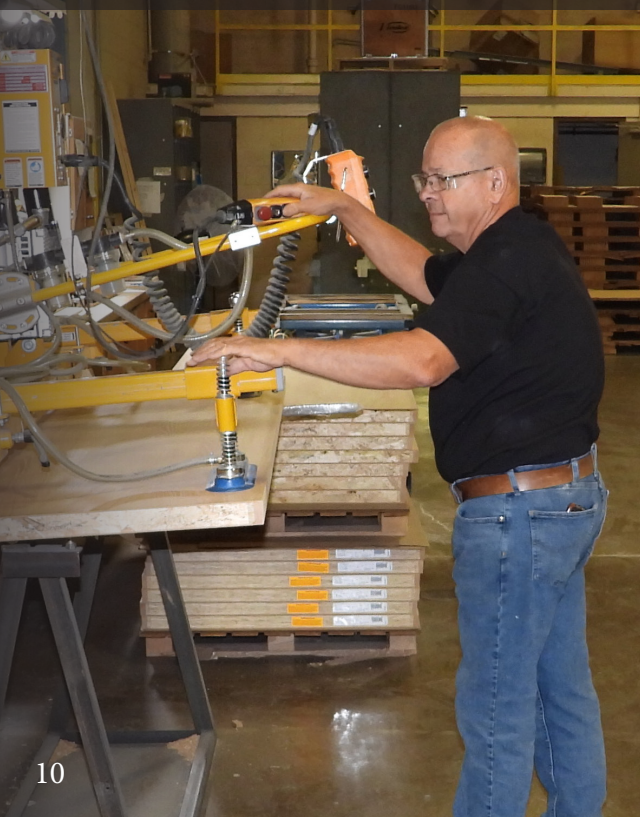
Glen Obry lines up a door to be cut on the mortising machine.
