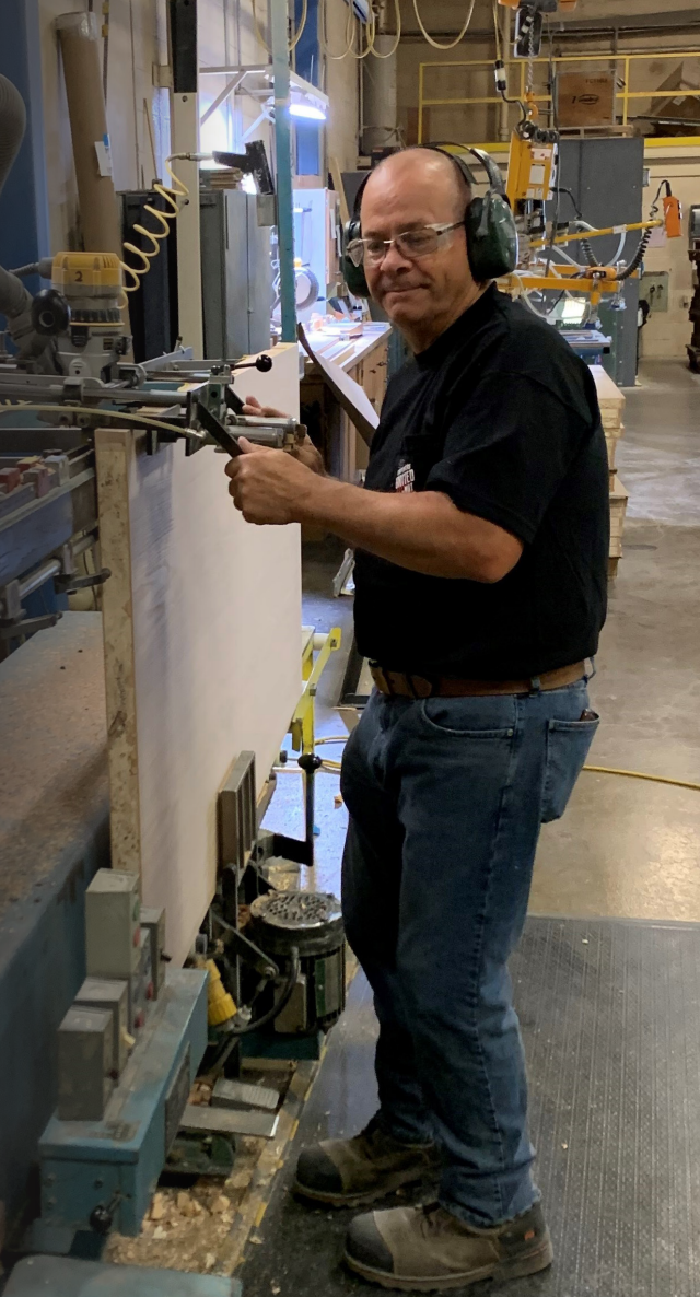
Glen Obry lines up a door to be cut on the mortising machine.
